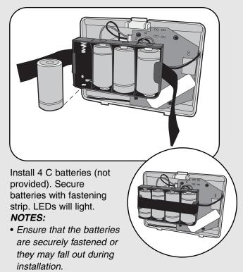
• To prevent damage to the circuit DO NOT use C size Lithium batteries.
